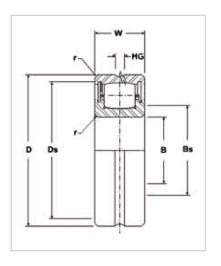
It is sealed single row spherical roller bearing. Single-row of large rollers result in increased dynamic load capacity and up to 100% greater misalignment of conventional double row spherical roller bearings. Sealing features are combined with the lip-wiping sealing function of an added contact seal, for applications where contamination conditions are particularly severe or where substantial amounts of moisture are present.
